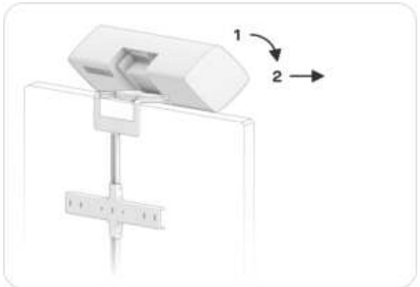
**Warning:** Do not leave Neat Bar in a max tilted position with the red indicator showing as it is not secured by the lock spring.
