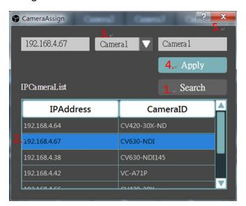
2.2.5. Select Camera to control from SelectCamera tab, Camera Control setting will be enabled.
