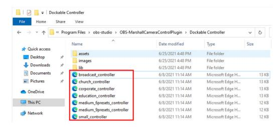
The controller samples in red box below are the dock type samples
