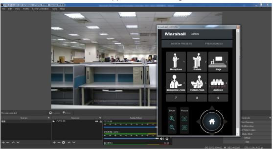
2.3.5. Click [PREFERENCES] to key in the IP address of the camera you would like to control and then push SAVE. After connecting to it, a window will appear and show camera is connected.
